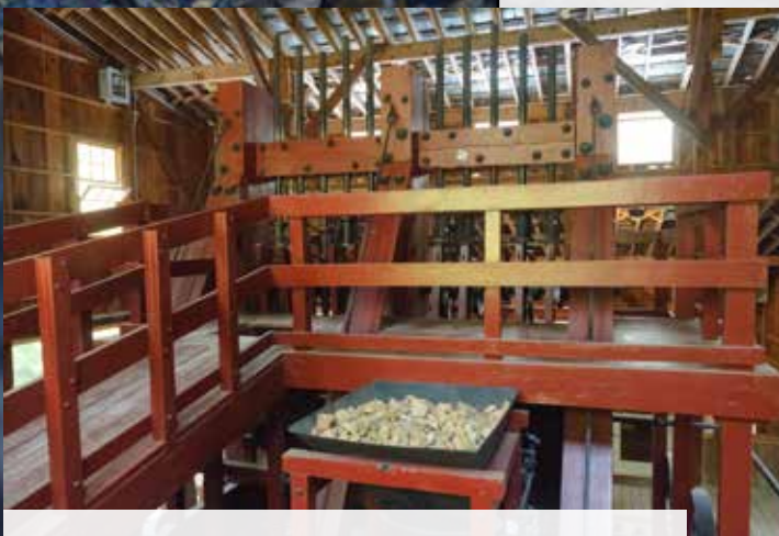
Top Left: Entrance to the Reed Gold Mine State Historic Site. Above: The 10-stamp mill is a machine that crushes material by pounding rather than grinding for extraction of the metallic ore. Right: A mine cart used for moving ore and materials.
